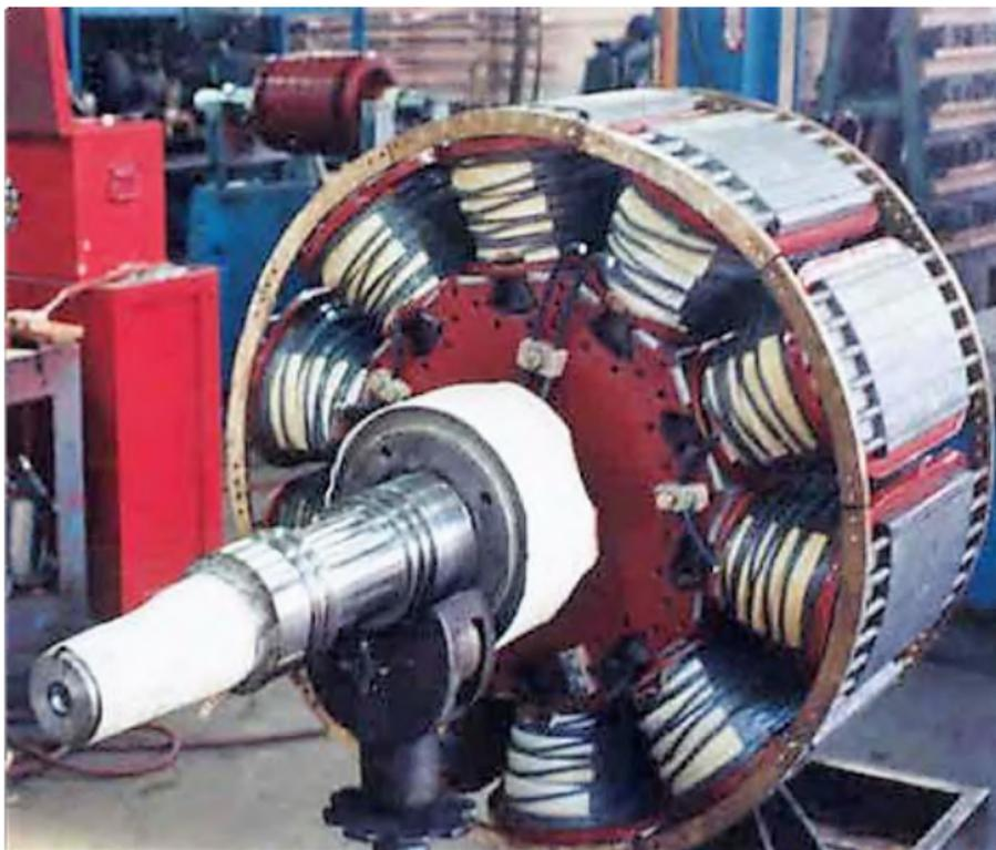
Figure 4 : Rotor of Alternator
