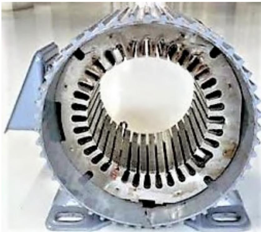
Figure 2 : Stator of Alternator
